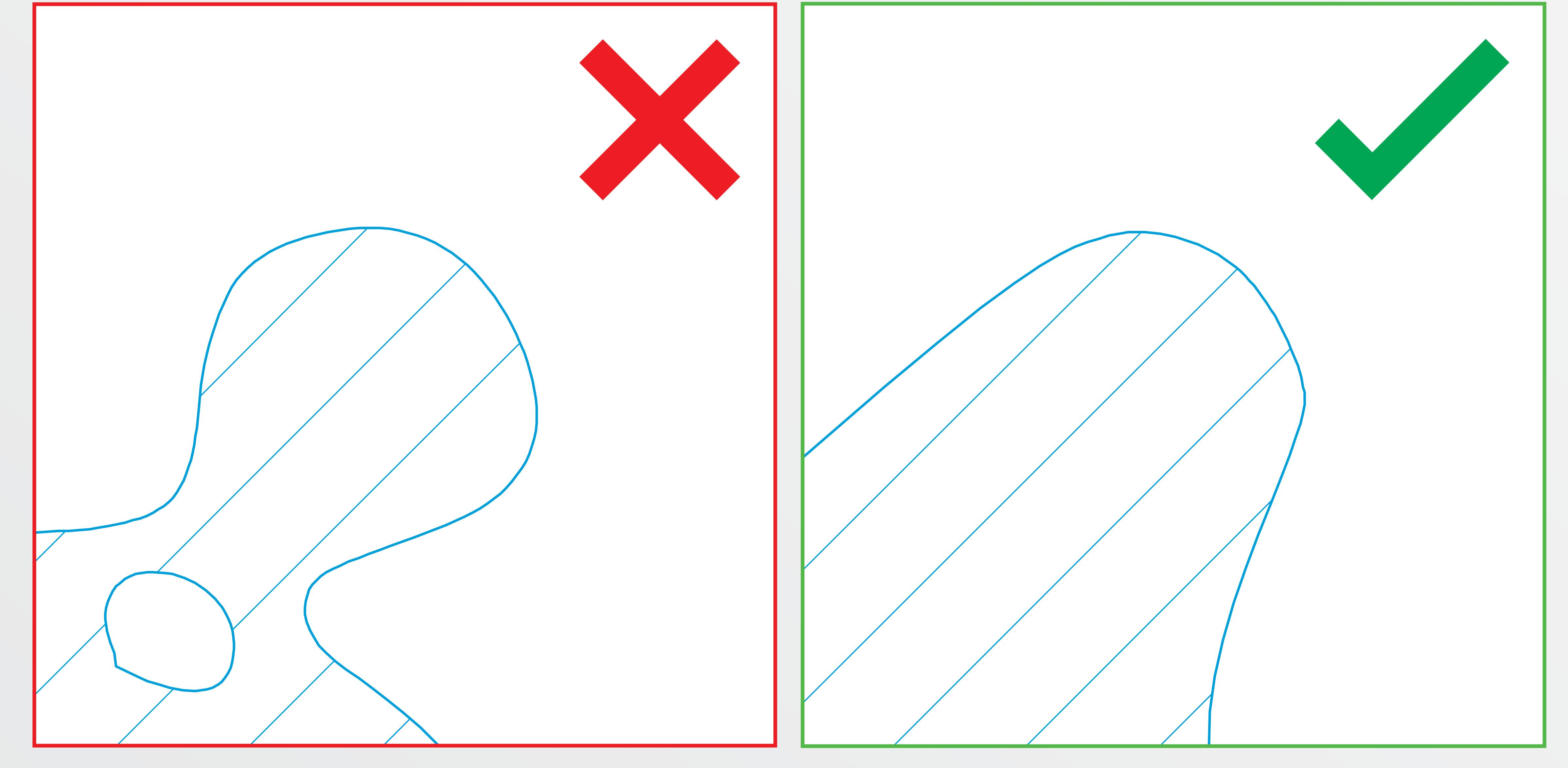
AVOID: NECKING, IT WILL MAKE THE MATERIAL WEAK ACROSS THE NARROWEST POINT AVOID: HOLES IN THE ARTWORK AS IT WILL MAKE THE MATERIAL WEAK AIM FOR: SHAPES THAT AREN'T WIDER AT THE EXTREMITIES
