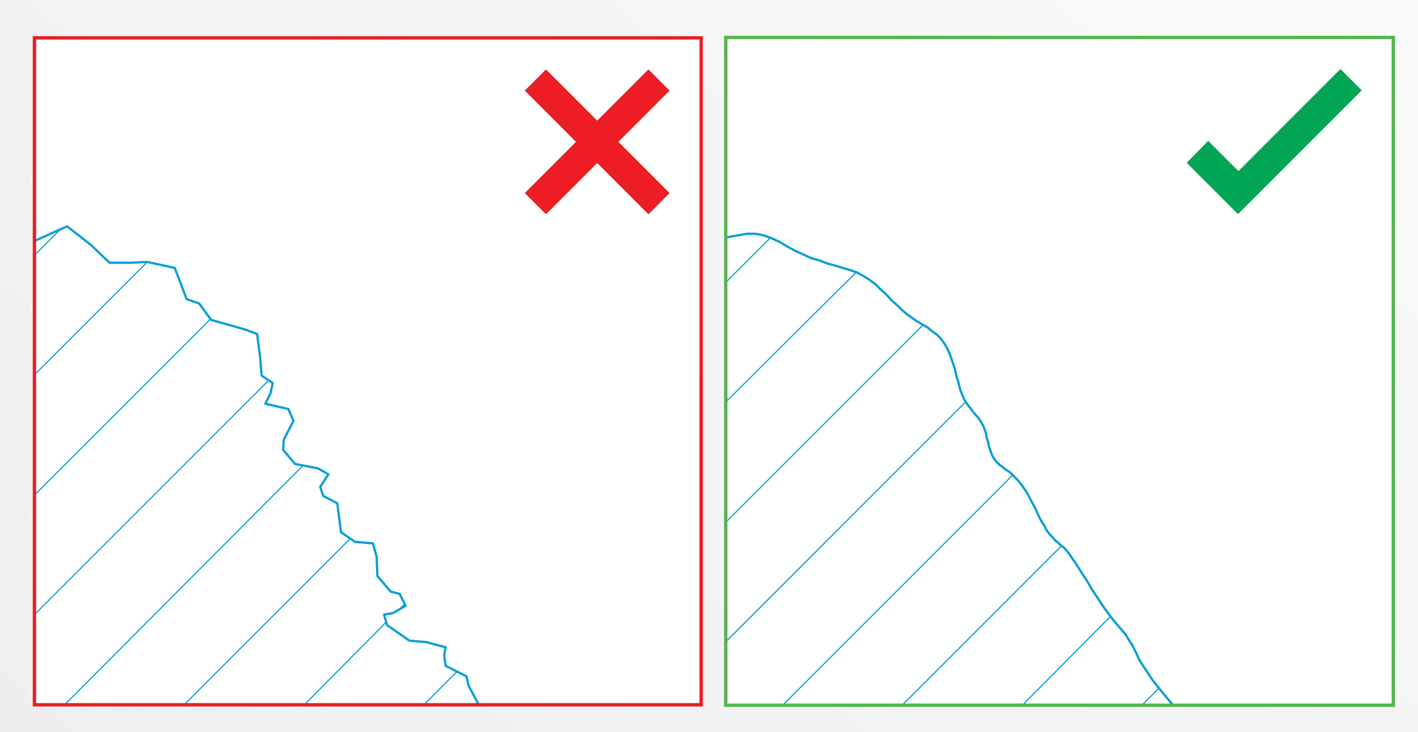
AVOID: COMPLEX AND JAGGED LINES, THESE CAN CREATE EASY LIFTING EDGES AIM FOR: SMOOTH FLOWING LINES, AS SIMPLE AS POSSIBLE
